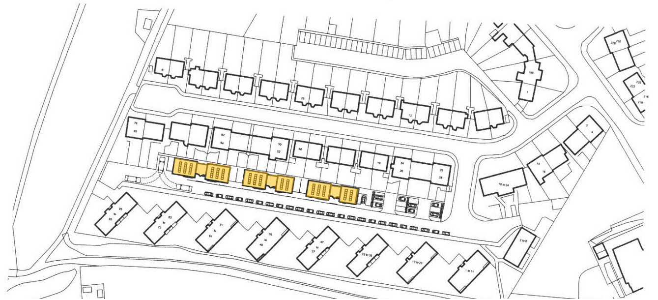
3No blocks with amenity space between and car parking to the south
